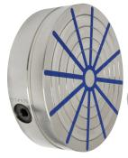
Neostar Chucks with Neodymium (rare earth) magnetic circuits are designed for holding rings and bearing races, as well as solid rounds. This chuck comes standard without center hole. An optional through hole can be provided upon request. Includes Allen key for actuation.
