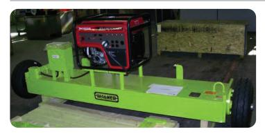
A towable electromagnetic sweeper design that is supplied with wheels, pneumatic tires, adjustable towbar, and parking stand. Stand folds up into the towbar when not in use. All units can be supplied with a heavy duty 115volt AC generator mounted to the top. Generators are powered by a 4 stroke OHV gasoline engine and are energized and de-energized using the 115 VAC "ON" – "OFF" switch on the generator. A remote switch on 20ft of cable is available upon request.
