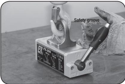
10. When you turn off, Ensure that the lifting magnet is completely switched off (indicator is also the Safety groove which must be completely visible again)
