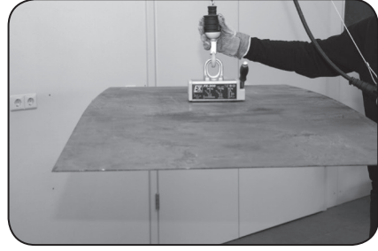
7. Run the lifting operation. Note that the lever of the lifting magnet must not be used as Hand guide
