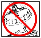
ALWAYS SET A MAGNET DOWN EASY Ease the magnet down onto the material. Repairs are costly and time-consuming.
