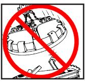
**KEEP TERMINAL BOX CLOSED** This keeps moisture away from the terminals and out of the magnet coil.
