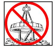
KEEP POWER OFF UNTIL THE MAGNET SETTLES ON THE LOAD Lift the load 2 to 3 inches then jar the load to ensure that adequate holding power is available.
