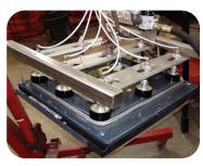
\*Destacking (Option DS): Required for applications destacking metal that is thin. See Chart. (available on TPL30 & TPLP50 only). The Destacking Option features a special magnetic circuit that is designed to destack sheets as thin as 0.030" (22 ga).
